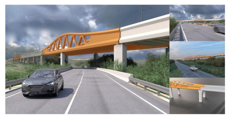
$Total\ length\ of\ 613\ m\ with\ 2\ stell\ truss\ sections\ over\ EX-A1\ and\ EX-108\ highways,\ and\ 3\ sections\ of\ concrete\ deck$
